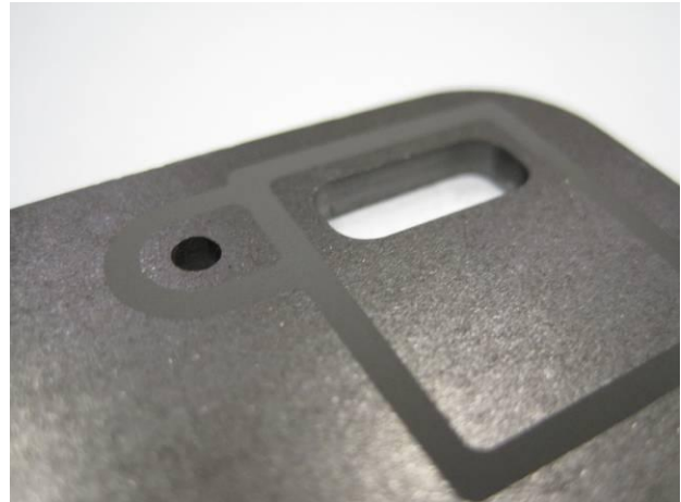
Figure 6. Screen Printed storage stable adhesive layer on a graphite composite bipolar plate
