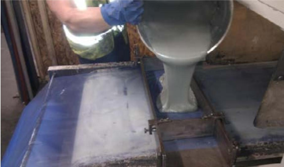
Figure 2. The phenolic resin/CSR/filler mix being poured into the “doctor box”
