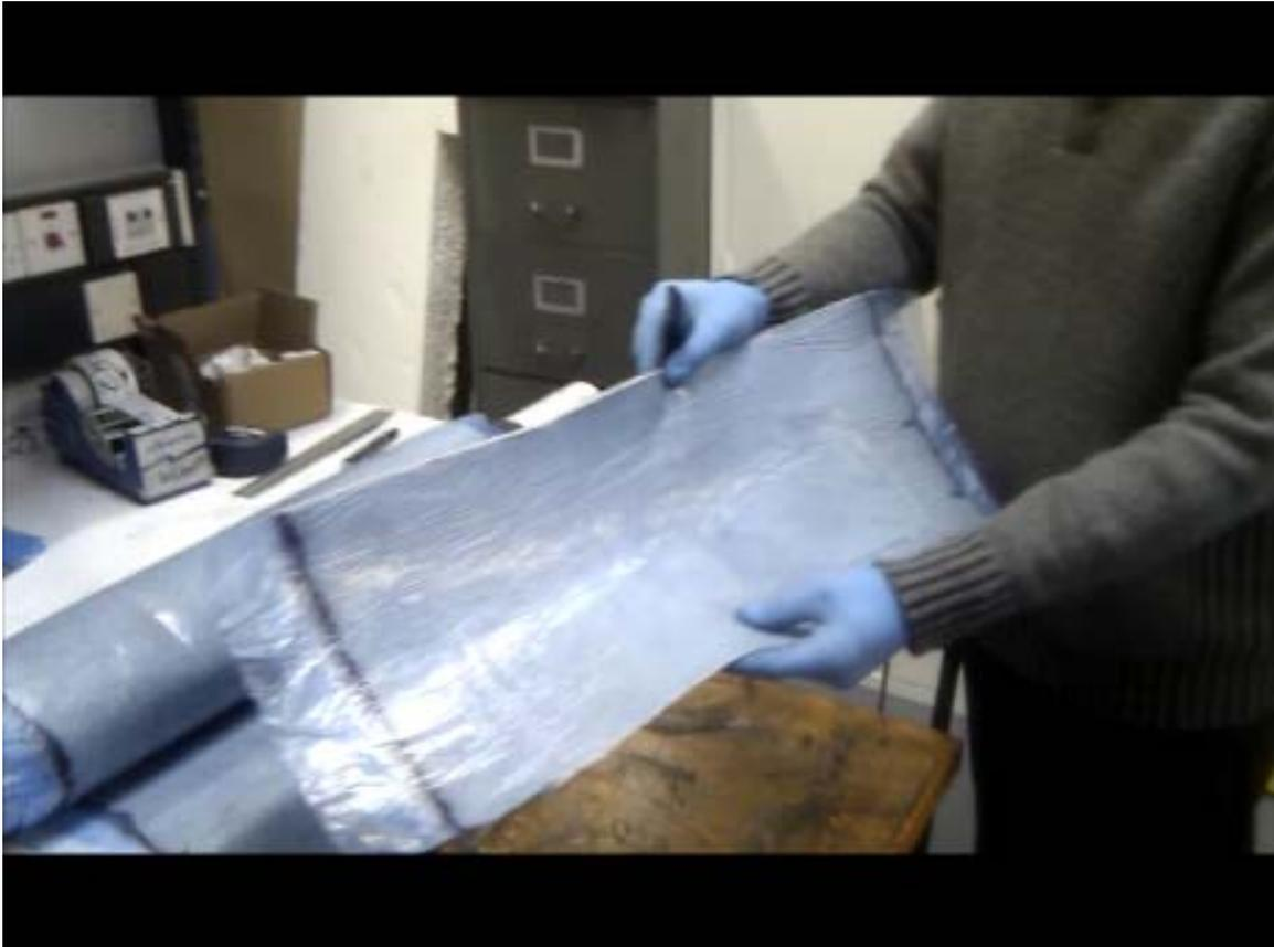
Figure 5. Thickened (matured) phenolic SMC sheet, cut and ready for moulding
