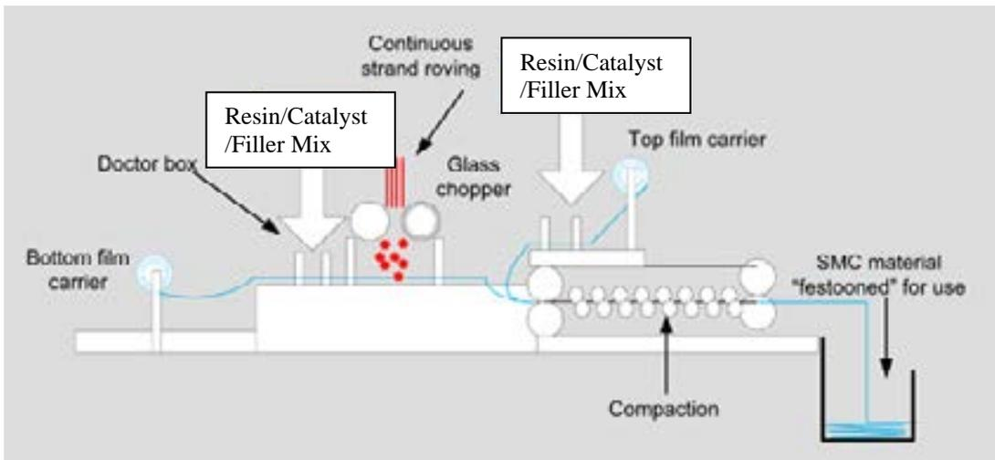
Figure 1. Sheet moulding compound production line
