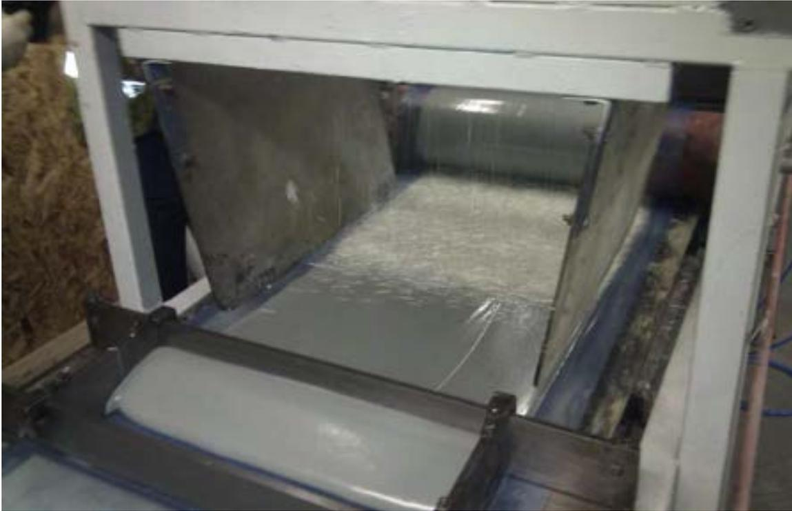
Figure 3. Chopped glass added to the bottom resin layer
