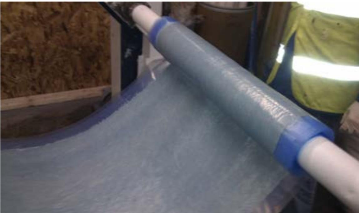
Figure 4. The phenolic SMC is formed into a roll and stored until thickened.
